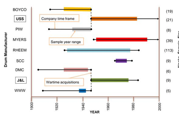
Figure 2. Representative sample drum year data from database plotted against historical drum manufacturer information.
